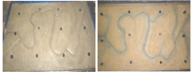
Fig.2 Change of soil bed by spreading gravel
