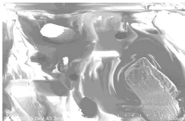
Fig. 1b. SEM micrograph of EFF/SCF/EFF hybrid composites.
